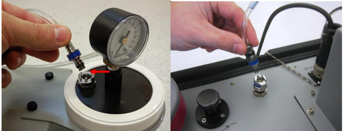
6. Install the Aerosol Mixer between the Aerosol Generator output and the Aerosol Mixer Port.
