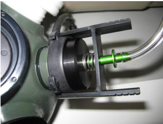
Example of EV Adapter installed on mask exhalation valve. This configuration may vary depending on the mask being tested.
