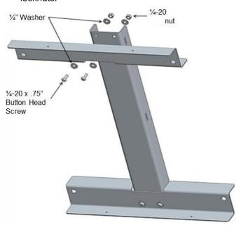
2. Attach the pole mount to 4 locations on the environmental enclosure using the provided 3/8" screws, washers, and nuts.
