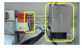
7. Plug the remaining Thermostat wire into the "+" side of the Heater Connector (left side of connector, Gray) as shown.
