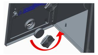
Remove vent plugs when weather conditions do not require use of the heater. Twist vent cover counter clockwise to remove vent plugs. Hand-tighten after removing plug.
