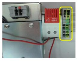
6. Install the Heater onto the DIN Rail and Plug into the two Phoenix Connectors just installed to the right of the Thermostat.
