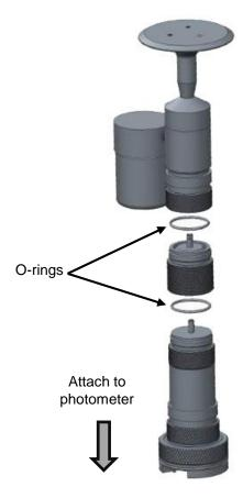
8. Attach column to Photometer inside Enclosure.
