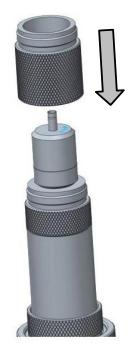
7. Re-attach water trap and Omni-directional Inlet Impactor Housing.
