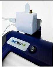
6. Connect the USB cable and RJ45 cable to the DustTrak Aerosol Monitor.
