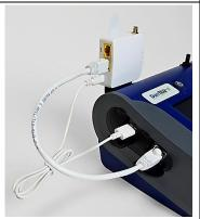
7. Screw the hinged antenna to the wireless router.
