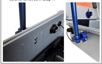
6. Using the nut that was removed in Step 4, attach the gland seal to the side of the enclosure. If needed, use an adjustable wrench to apply a small amount additional of torque to the nut.
