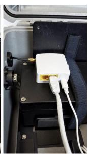
11. Connect the antenna cable to the router.
