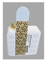
Remove black liner and attach wireless router to the front plate of the DustTrak Aerosol Monitor as shown.
