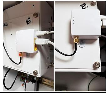
Connect the DustTrak Aerosol Monitor's power cable to the power supply mounted on the DIN Rail.
