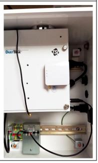
9. Connect USB cable, RJ45 cable and antenna cable to the wireless router. Connect the RJ45 cable to LAN port on the router.
