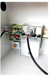
11. Connect AC power cord to the side of the enclosure.
