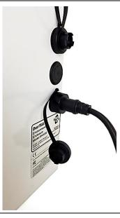
12. Connect the other end of the power cord to an AC main terminal. The blue light on the DustTrak monitor will illuminate, indicating the instrument has power. After two (2) minutes, the red and green LEDs on the wireless router will also illuminate.
