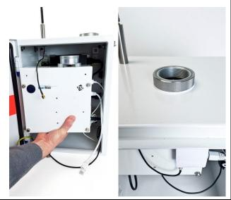
Remove blue liner and attach a 3M<sup>™</sup> Command<sup>™</sup> brand strip to the back of the wireless router. Be sure not to cover the vent holes. Refer to the Command<sup>™</sup> brand strip box for additional instructions.
