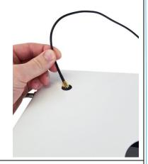
2. Secure antenna post to enclosure with retaining nut. Hand-tighten.
