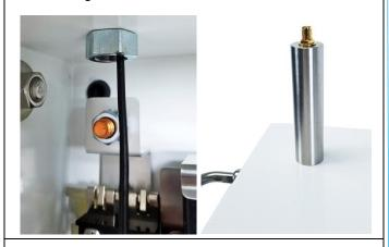
Fasten 1dB hinged antenna to bulkhead on top of the antenna post. Hand-tighten only.
