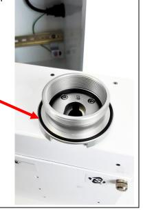
6. Install the DustTrak Aerosol Monitor into the Environmental Enclosure. Be sure to place antenna cable over the top of the instrument. Secure to enclosure using the retaining ring and white plastic spacer that was included in the Omni-Direction Inlet kit. Refer to the Environmental Enclosure manual for additional DustTrak monitor installation instructions.
