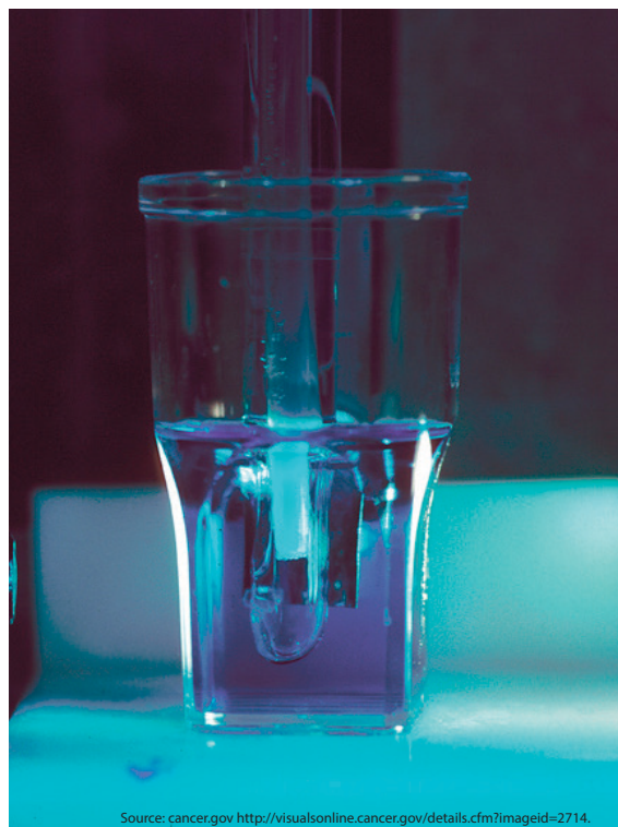
The Coulter Counter, shown here counting cells in solution, is an indirect volumetric particle analysis method.
