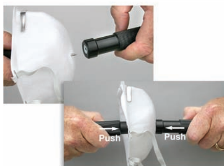
Step 4: On the outside of the respirator, align the push nut tool over the end of the exposed point. Hold the tools in-line with each other and firmly push them together as far as possible.
