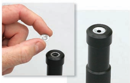
Step 2: Load a push nut onto the magnetic push nut tool.
