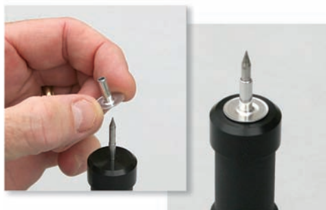
Step 1: Load a sample probe onto the piercing tool.
