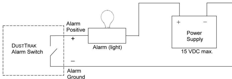
Since applications of this function will vary, TSI supplies only the output cable (part no. 801652). The output cable is labeled with the pin-out wiring diagram. The user is responsible for all additional equipment needed for making connections to their own equipment.
