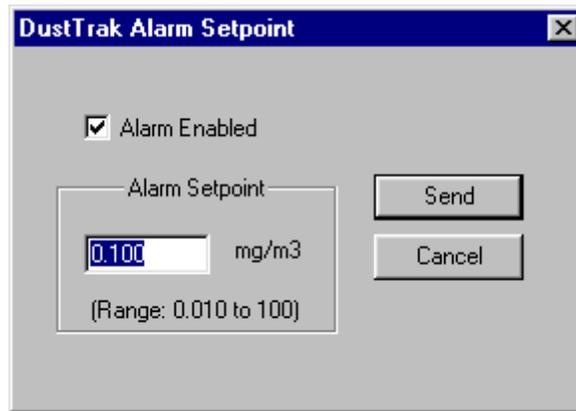
4. Turn “On” the alarm function by checking the “Alarm Enabled” check box. Enter a value within the acceptable range. In this example, the DUSTTRAK™ monitor is programmed to a setting of “0.100 mg/m<sup>3</sup>.” Press the **Send** button, to program the instrument.
