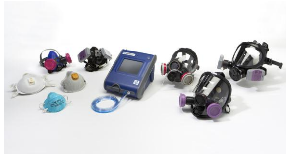
TSI Model 8038 PORTACOUNT® PRO+ Respirator Fit Tester with N95-Companion™ technology
