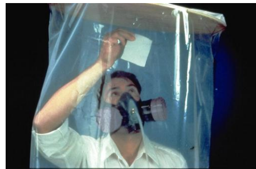
Banana oil fit test
