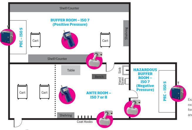
Example of a clean room floor plan suitable for high-risk level CSPs and Hazardous Drugs
