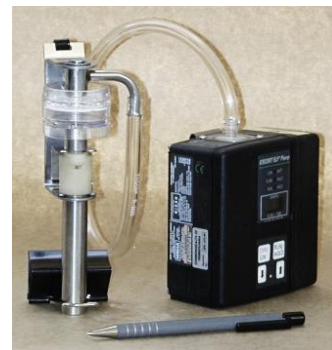
Sample Pump with Respirable Silica Sampling Train
