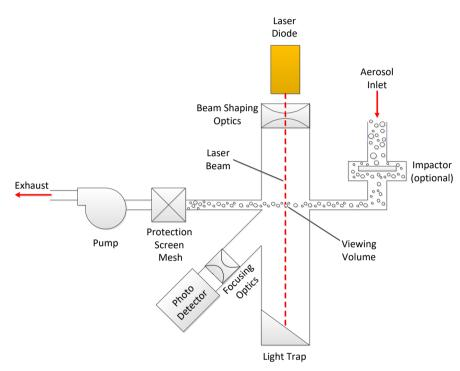
constant to yield factory calibrated mass concentration. The internal calibration constant is determined from the ratio of the voltage response of the SidePak<sup>™</sup> AM520/AM520i monitor to the known mass concentration of the calibration test aerosol (A1 Test Dust).
