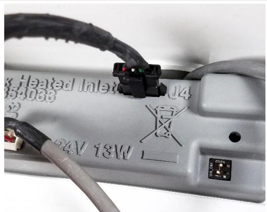
14. If using a Thiamis 1000 Node, route the other side of the cable to the power input on the Thiamis node (green connector).
