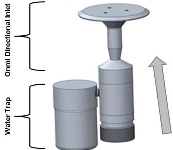
2. Unscrew the PM2.5 or PM10 impactor to access the impactor plate as it comes pre-assembled from the factory.
