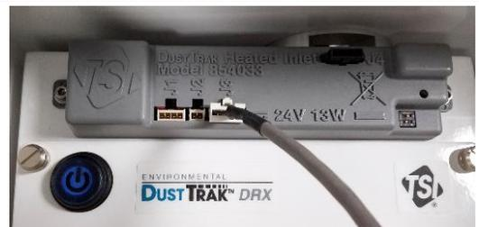
6. Attach the two larger (gray) connectors to side of the photometer.
