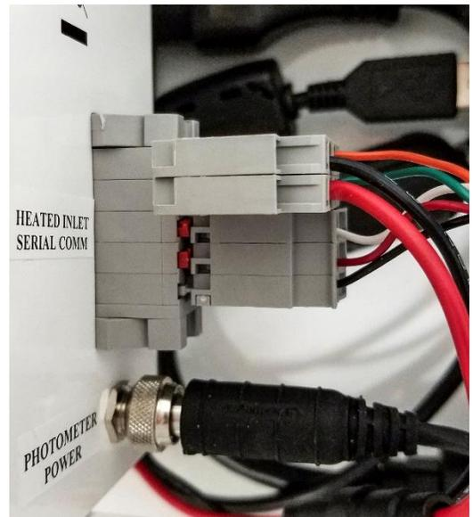
7. Attach the two smaller (white) connectors to the Power/Communication inputs (J1 and J2) of the heated inlet control module (RH/Temp Sensor Cable J3 is not shown for clarity).
