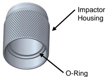
7. Thread (hand-tighten) the impactor housing with O-ring onto the heated inlet column.
