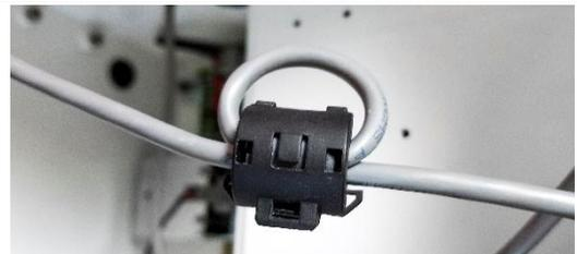
13. Attach heated inlet cable to heated inlet control module (J4).
