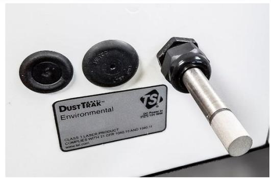
4. Attach the sun shield to the top of the RH/Temp Sensor as shown. Sun Shield should not touch sintered cap of RH/Temp Probe.
