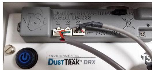
8. Install O-ring and route cable through the mounting ring. Pull excess cable through to prevent pinching of cable when inlet column is installed.
