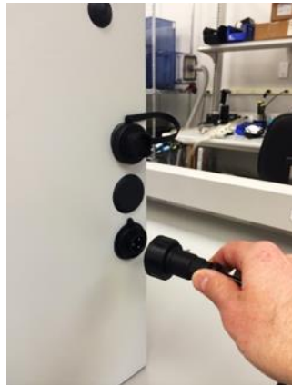
Figure 20: DustTrak Power Connection ( left ). Final connection to exterior AC power source (DC power source will use 2-pin connector on left side of enclosure – right )
