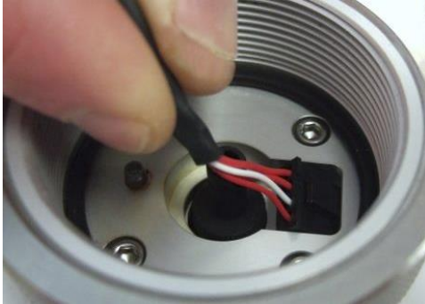
Figure 27: Removing heated inlet assembly
