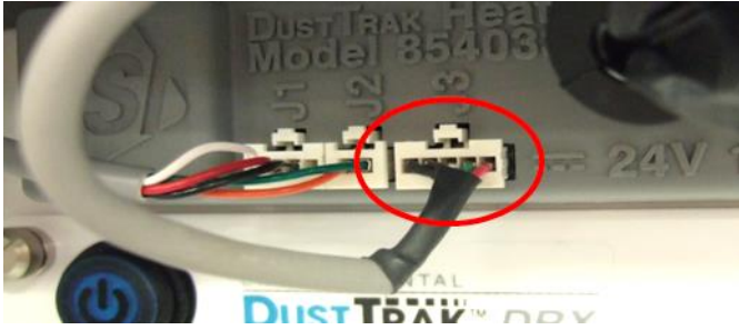
Figure 29: Disconnecting temperature/humidity cable
