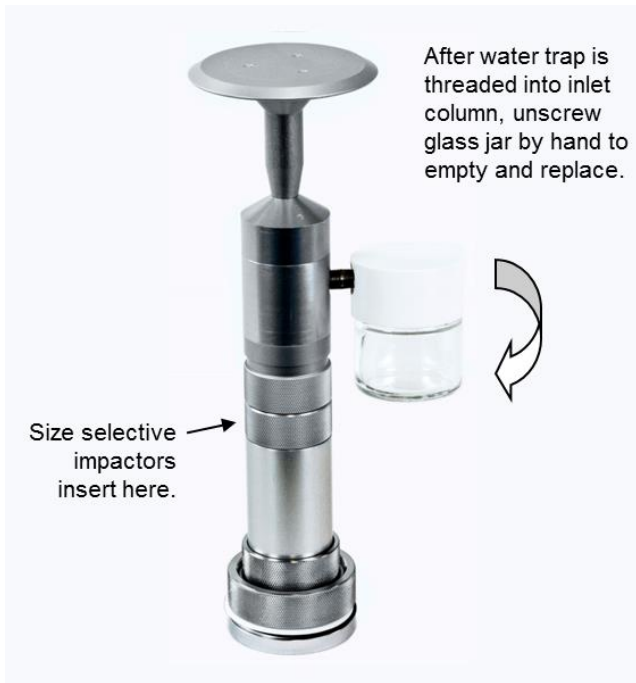
Figure 18: Removal of glass jar from flow stack
