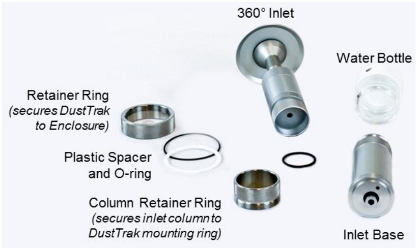
Figure 14: Inlet column parts
