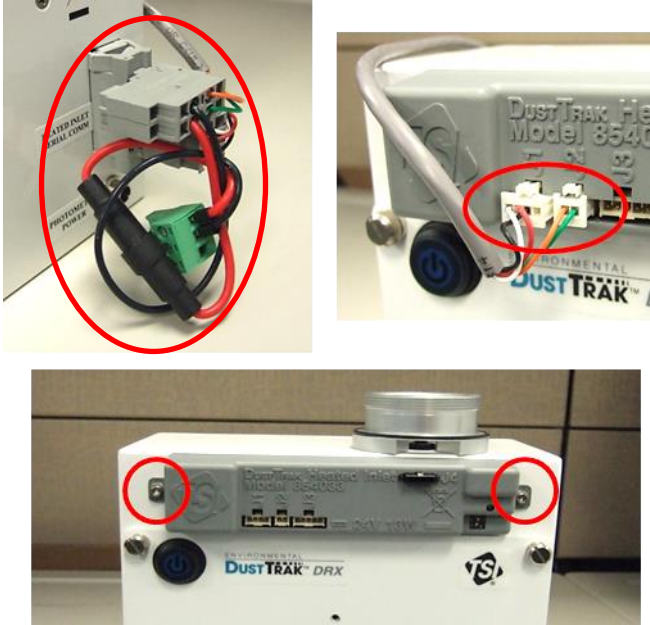
Figure 31: Removing cables and heated inlet controller
