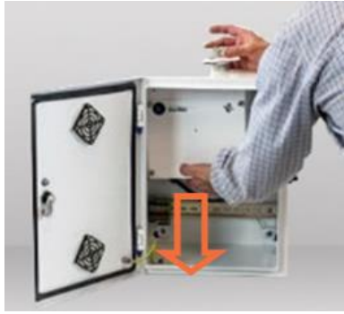
Figure 25: (a) Heated inlet cable; (b) remove retainer ring and lower photometer
