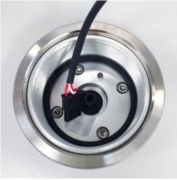
Figure 25: (a) Heated inlet cable; (b) remove retainer ring and lower photometer
