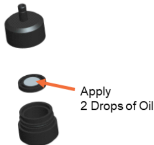
Figure 19: Apply two drops of oil to impactor plate
