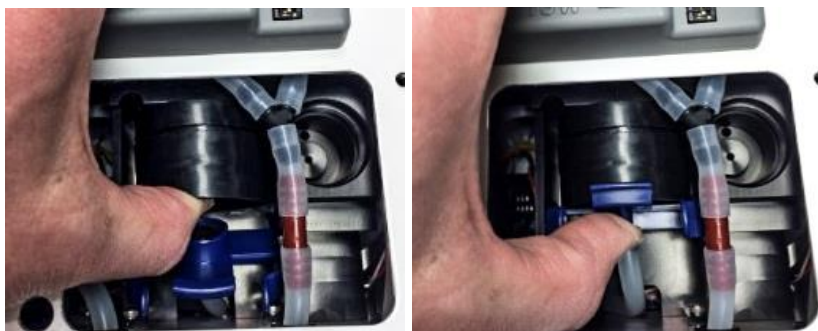
Figure 35: Snap cassette securely into inlet port
