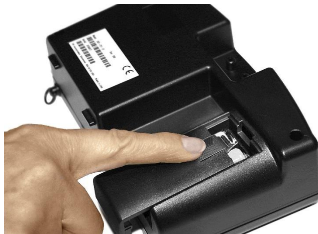
Figure 5: Battery Cover Removal
