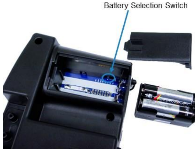
Figure 6: Location of Battery Type Selector Switch
