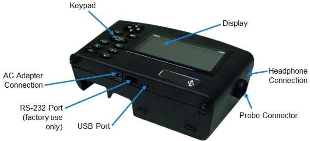
Figure 1: Features of the Model 8715/8380 Micromanometer, Front View
