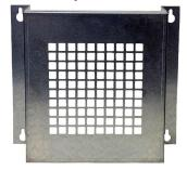
The metal protective guard is made of heavy duty metal and helps to protect against abrasive damage, theft or vandalism to the transmitter. It is made from 16-gauge galvanized steel and has  $\frac{1}{2}$ " (13 mm) square openings in the front to allow gas and air to flow through to the sensor. With only four slotted mounting holes, installation and removal for gas detector servicing is easy.
