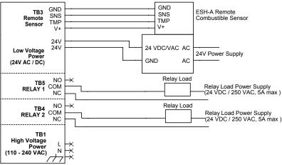
A class 2 or better transformer must be used. The stated max current draw of the SCC in this mode is 0.5 A.
