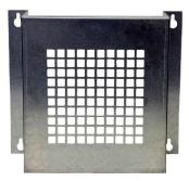
The metal protective guard is made of heavy duty metal and helps to protect against abrasive damage, theft or vandalism to the controller. It is made from 16-gauge galvanized steel and has 13 mm ( $\frac{1}{2}''$ ) square openings in the front to allow gas and air to flow through to the sensor. With only four slotted mounting holes, installation and removal for equipment servicing is easy.
