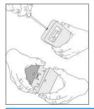
**NOTE:** Do not apply caulking or other material around the gas detector base. The gas detector relies on air exchange through the spaces between the base and the gas detector housing. Do not obstruct the small gap around the housing and the base with any material.
