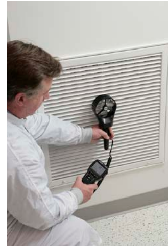
Rotating vane measuring an outlet
