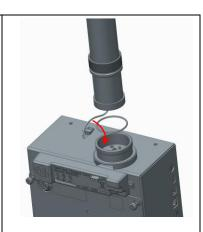
13. Match pin on inlet column with hole on top of retainer ring to properly align the inlet column (enclosure not shown for clarity).
