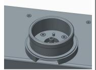
4. Push out elastic plug and install RH/Temp Sensor Gland to side of environmental enclosure.
