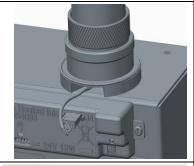
14. Attach ferrite to cable with one wrap of the cable and snap the ferrite together (enclosure not shown for clarity).
