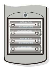
After replacing the batteries, the date, time, baud rate, type of probe, printing interval, logging parameters must be set again: in order to simplify the operation, on insertion of the new batteries the instrument turns on automatically and requests these parameters in sequence. To go to the next item press ENTER; to return to measurement mode, press MENU.
