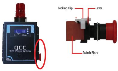
An optional emergency stop, push button switch that is factory installed on the side of the QCC enclosure. Allows manual shutdown of equipment in the event of an emergency such as a gas leak. Ideal for refrigeration applications; when combined with the Top Mounted Strobe, meets B52 code requirements.
