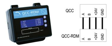
Either TB2 or TB3 can be used to connect the QCC to the QCC-RDM. Both are Modbus® connections. The QCC-RDM will automatically broadcast the display information to Modbus® ID 253. This is the common Modbus® ID for all QCC-RDMs on the network and is used to listen for broadcasts from the QCC and receive screen updates from the QCC. The read and write default QCC-RDM Modbus® ID is 230.
