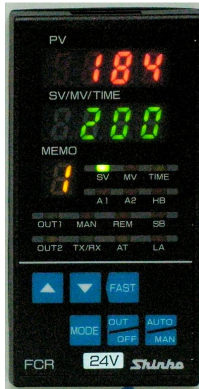
Figure 4-7 Thermal Conditioner Temperature Control.
