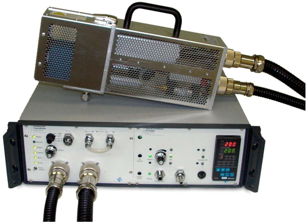
Figure 1-2 Model 379020A-30 Thermodiluter Control Unit, Connections, and Thermodiluter Head and Thermal Conditioner Air Supply
