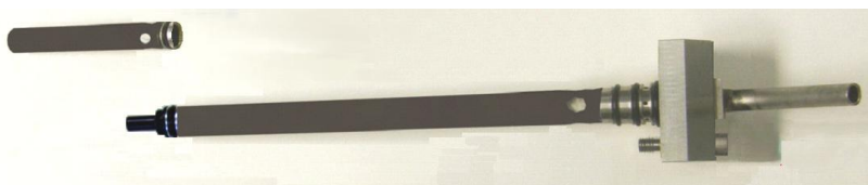
Figure 9-5 Wick Cartridge Growth tube and Conditioner shown separated.
