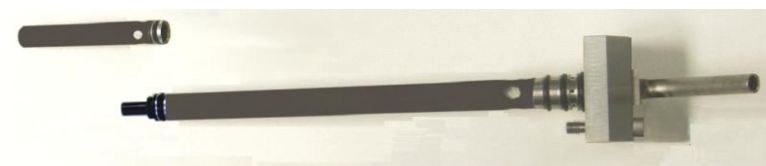
Figure 9-5 Wick Cartridge, Growth Tube separated from Conditioner
