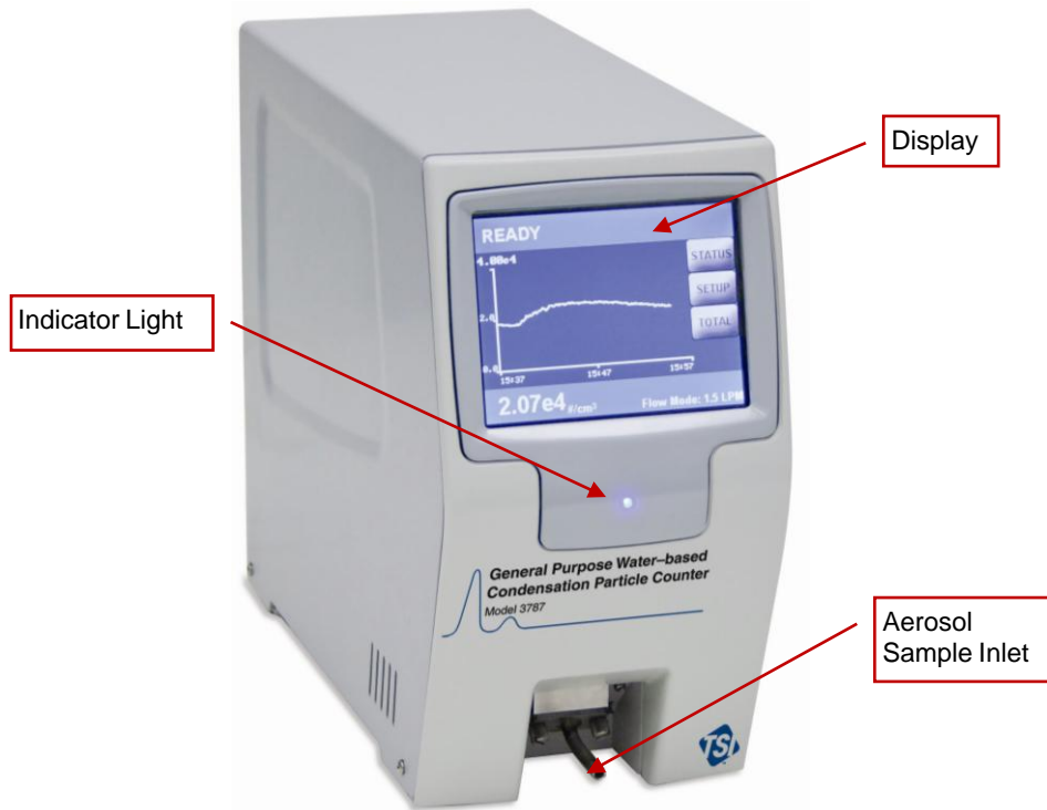
Figure 4-1 General Purpose Water-based Condensation Particle Counter Front Panel
