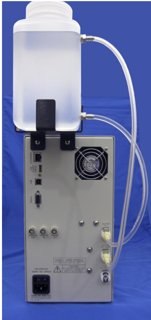
Figure 2-2 Attaching the Water Bottle Tubing Connections
