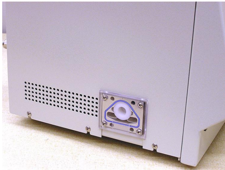
Figure 3-4 Left Side Panel Showing Butanol Reservoir and Saturator Wick
