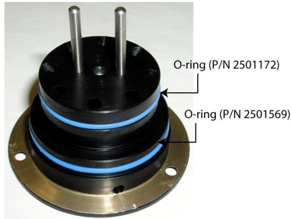
Figure 8-7 O-Rings on Saturator Base (P/N 2501172 and 2501569)
