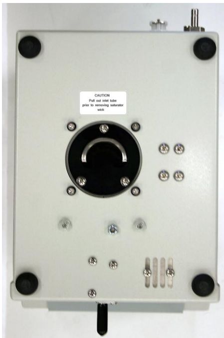
Figure 3-5 Bottom Panel Showing Removable Saturator Base
