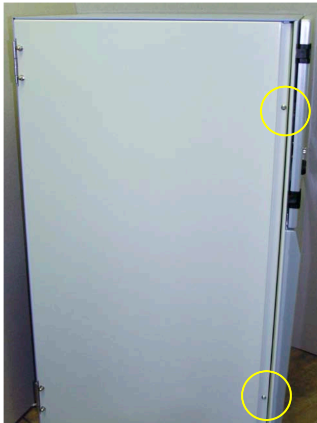
Figure 6-5 Model 3031 Left Door Showing Retaining Screws
