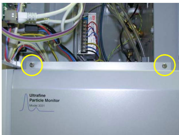
Figure 6-3 Location of Top Screws on Front Bottom Door
