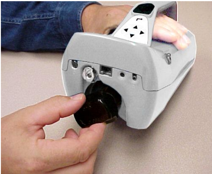
Figure 2-6: Insert Alcohol Cartridge into Condensation Particle Counter
