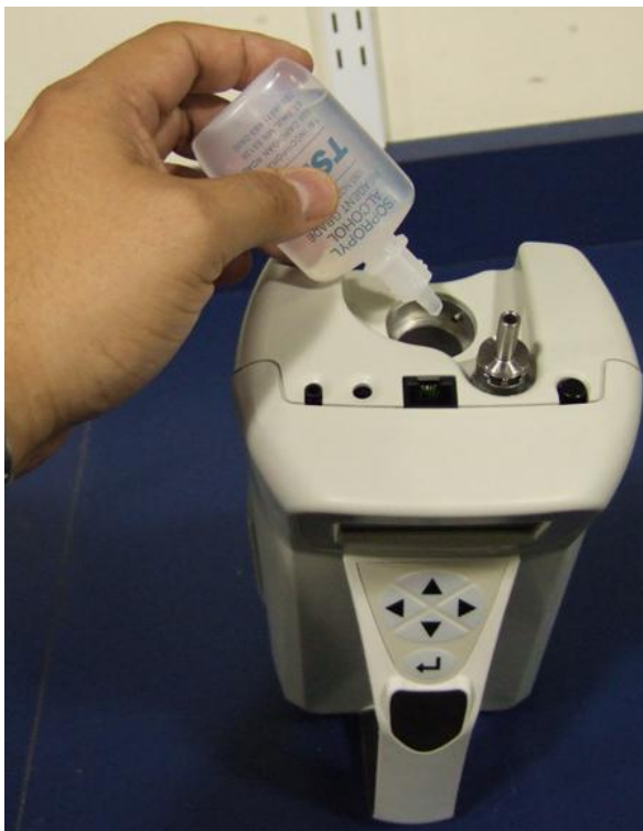
Figure 5-2: Drip 3 to 4 Drops of Alcohol into the Cartridge Cavity
