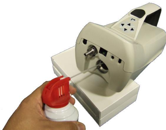
Figure 5-1: Apply 2 or 3 Bursts of Gas into CPC
