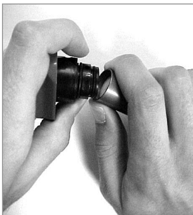
Figure 4-1: Snap Apart Cartridge
