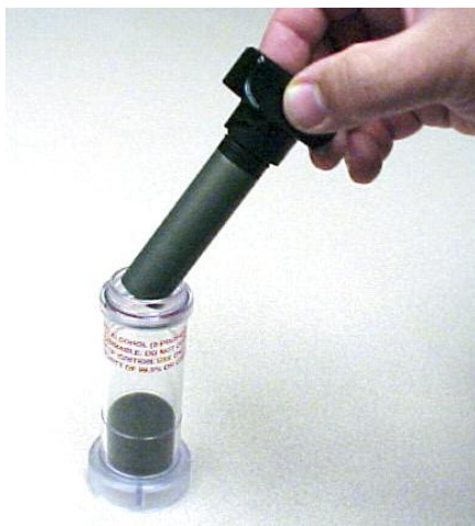
Figure 2-5: Insert Alcohol Cartridge into Fill Capsule
