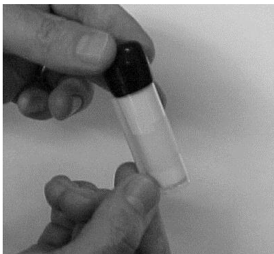
Figure 4-2: Remove Wick and Screen Using Dowel
