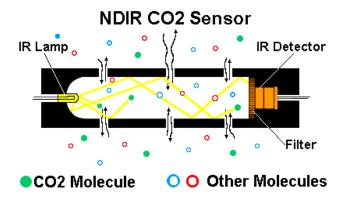
As shown in the figure, gas molecules diffuse into the sensing chamber. The IR light is directed through the sensing chamber towards the detector. The detector has a filter in front of it which eliminates all light except the  $4.26 \, \mu m$  wavelength that  $CO_2$  molecules can absorb. Since other gas molecules do not absorb light at this wavelength, only the  $CO_2$  molecules affect the amount of light reaching the detector.
