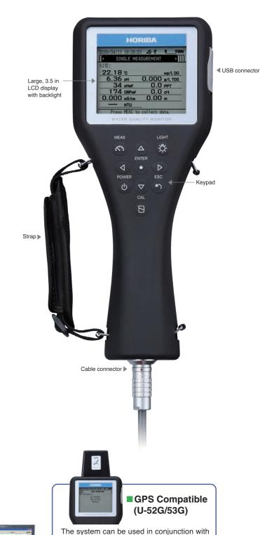
the Global Positioning System (GPS) to record latitude, longitude, and other location data for individual measurements. This is particularly useful for environmental surveys.
