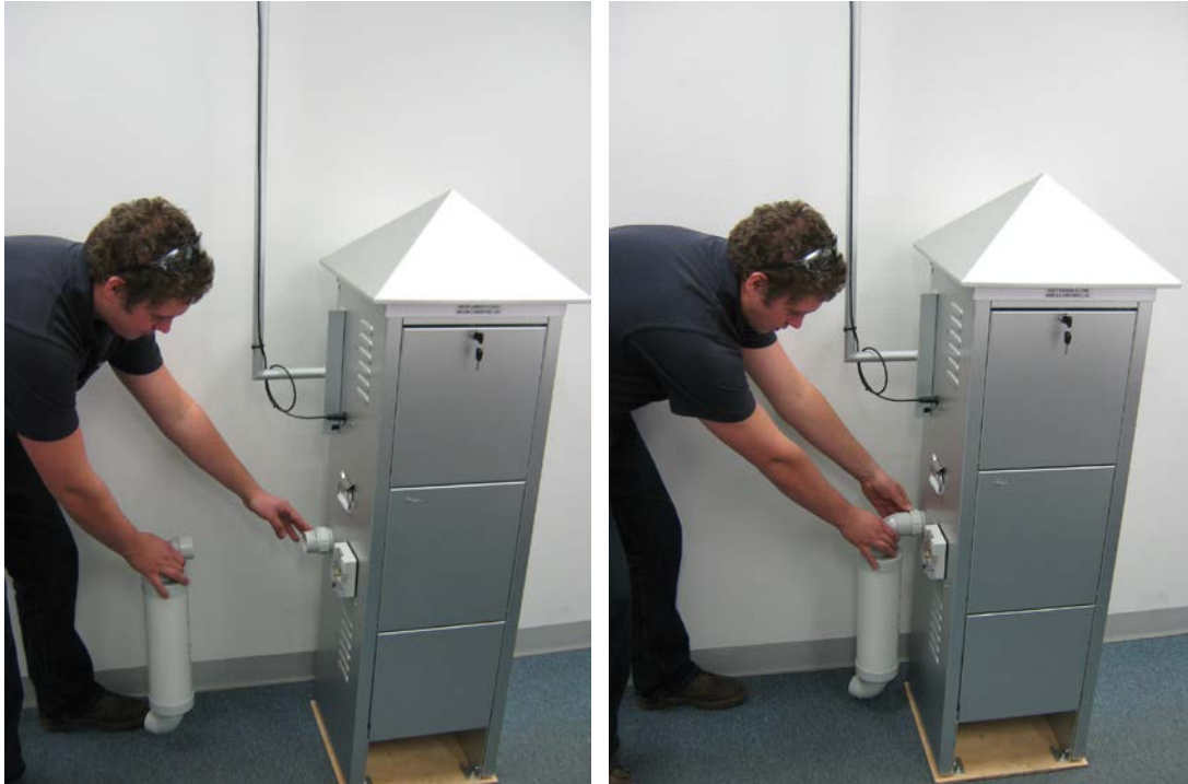
Figure 7 – Installing the optional muffler
