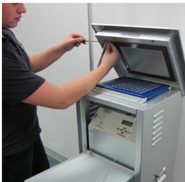
Figure 6 – Attaching the support stay
