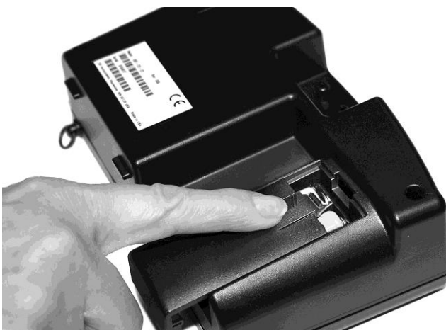
Figure 5 Battery Cover Removal
