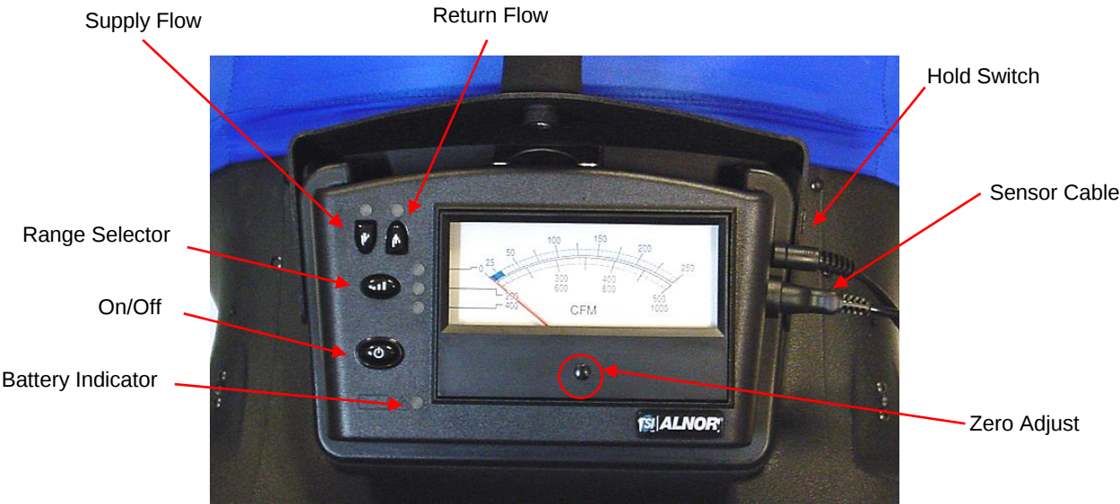
Figure 7 Analog Meter Components
