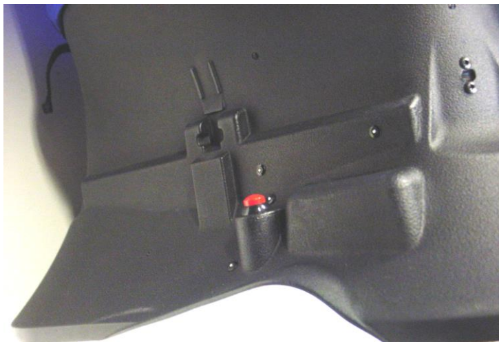
Figure 8 Red Hold Switch Location
