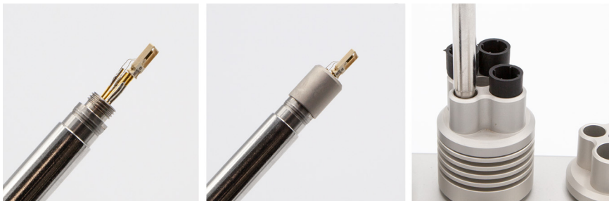
Figure 39 HMP5 calibration with HMK15 using 211302SP adapter
