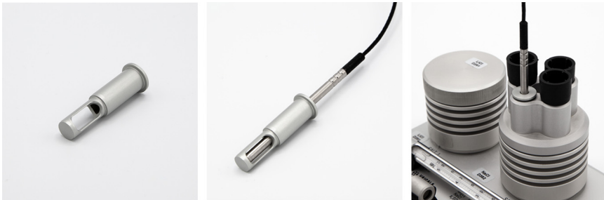
Figure 40 Using HMP9 calibration adapter with HMK15
