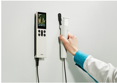
Figure 2 Using magnetic hangers to attach Indigo80 and GMP252 to metallic surface
