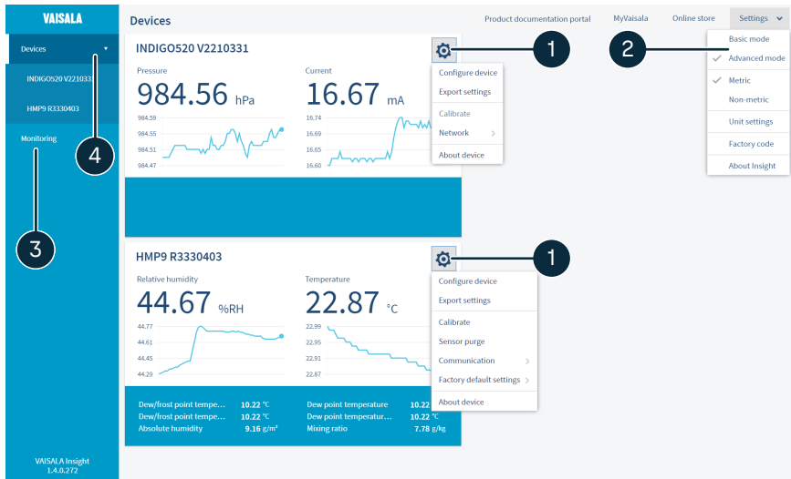
Figure 78 Insight software main view with transmitter and connected probe
