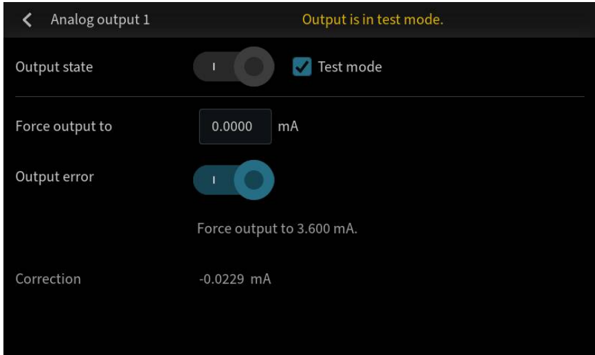
Figure 57 Analog output 1 Test mode on touchscreen
