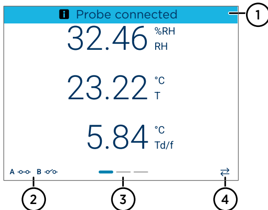
Figure 3 Indigo200 display with notification message, relay icons, 3 parameters, and USB connection icon
