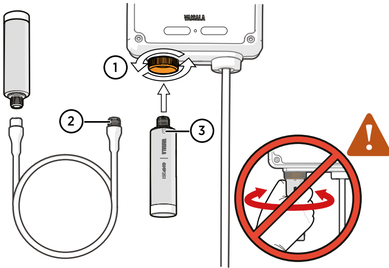
Figure 5 Attaching probes and cables to Indigo200
