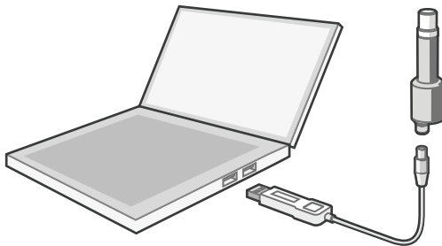
Figure 22 Connecting probe to Insight
