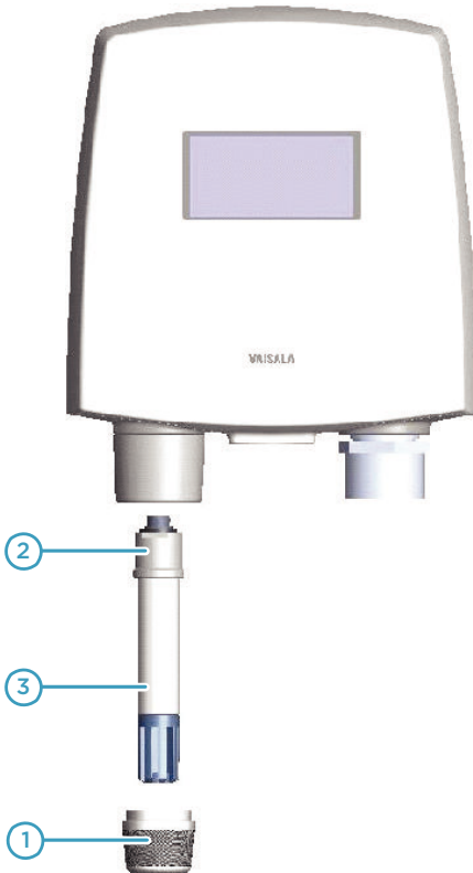
Figure 13 Removing the Humidity Probe (Fixed Probe Model)
