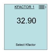
Make adjustments to the indicated value with the  $\triangle$  or  $\nabla$  keys and press  $\leftarrow$  to accept, or enter the **Select Duct** or Select **Kfactor** menu to choose a different pre-programmed flow value or dimension depending on instrument model:
