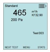
When measuring **Flow** as the **Primary** measurement, the parameters can be quickly changed by pressing the  $\triangle$  or  $\nabla$  key while on the main measurement screen:
