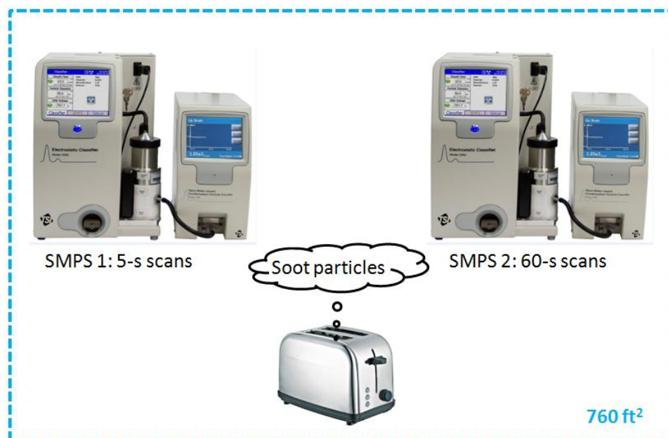
Figure 1: SMPS spectrometer set-up for fast scanning measurements of soot aerosol.
