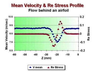
From these measurements all the higher order statistics, including Reynolds stress values, were calculated. The FlowSizer™ system software package, included with the FSA signal processor, is used for data acquisition and analysis. Optional XPD60 beam expanders can be used when the measurement distance (stand-off) is greater than about 500mm. This will maintain a favorable f# and this signal quality and data rates will be high.
