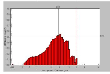
The aerodynamic size distribution of the suspension pMDI again is a non-Gaussian one that indicates two modes. The 3D-plot reveals this even more clearly: one mode is of a very narrow, submicrometer aerodynamic size with a wide light scattering range, while the other mode ranges from 1 to ~6  $\mu$ m in aerodynamic size but only a small scatter around an intensity of about 10.
