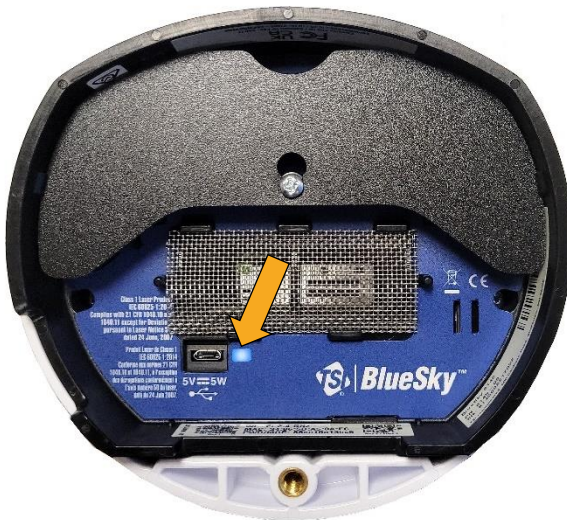
Figure 22: Connect to internet – LED solid blue ( power cord not shown for clarity )
