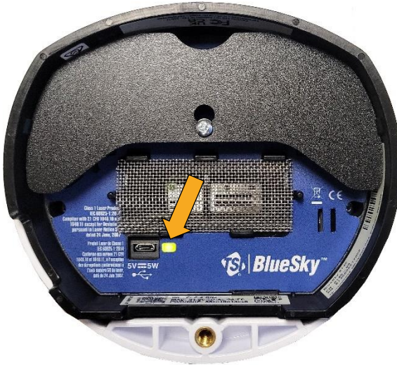
Figure 7: Set up mode – LED pulsing yellow (power cord not shown for clarity)
