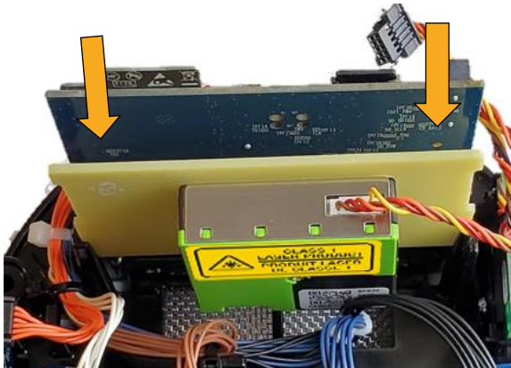
Figure 37: Install new sensor
