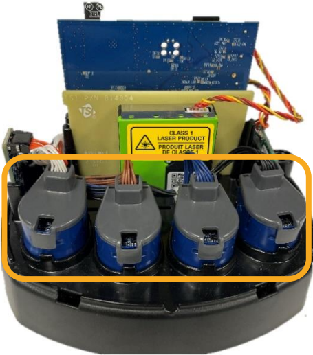
Figure 38: Replace electrochemical sensors
