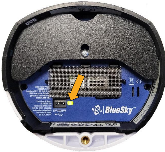
Figure 21: Start-up sequence starts again - LED pulsing yellow ( power cord not shown for clarity )
