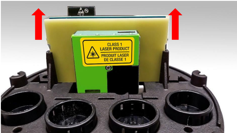
Figure 27: Replacing PM sensor
